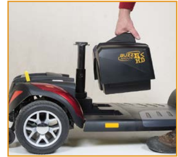
Step 2: Pull out the battery pack!
