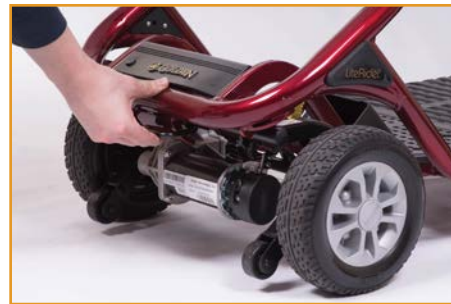
To separate the rear transaxle from the frame, squeeze the release lever located on the underside of the frame
